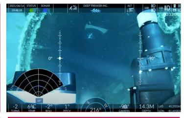
Precision sonar equipment for location and object detection
